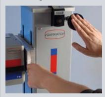
Push the hand wheel to unlock the height adjustment. The quick adjustment is activated. Position the marking head with the handhold above the part to be marked approximately.
