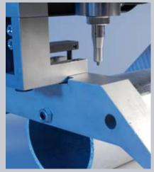
**Prism stop** For the application with round parts to be marked. Safe hold at marking. Fast and simple flange mount.
