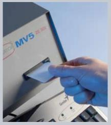
**Card reader insert** Simple definition of access authorisations and comfortable administration of marking files by a memory card. At the front of the central control unit.
