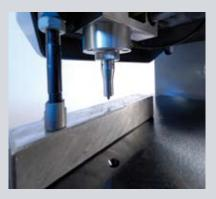
2. Set the required pin distance by the height detector and trim the distance by turning the hand wheel.
