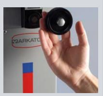
3. Lock the height adjustment by pulling the hand wheel. Hold the part to be marked under the positioned pin and start marking! The total required time here for is under 10 seconds!
